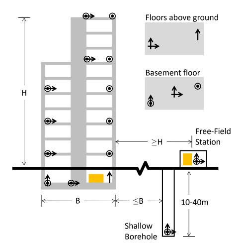
Data from a building with this level of instrumentation will enable engineers to accurately estimate input ground motions, spectral accelerations, effects of soil-structure interaction, overturning, interstory drifts, torsional effects, modal properties (periods, damping ratios, mode shapes), and peak floor accelerations, velocities, and displacements.
