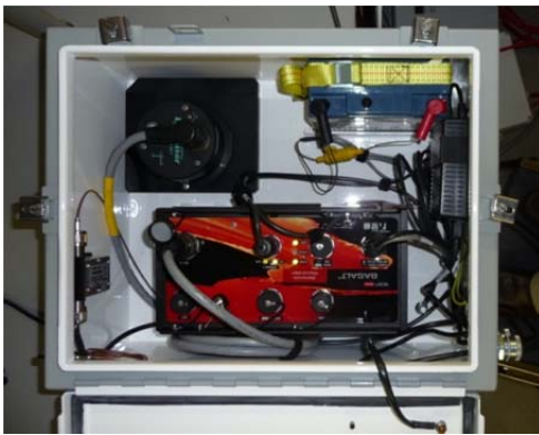
Figure 3. NEMA4 enclosure with Basalt, Battery, AC Charger, Episensor, and sensor plate
