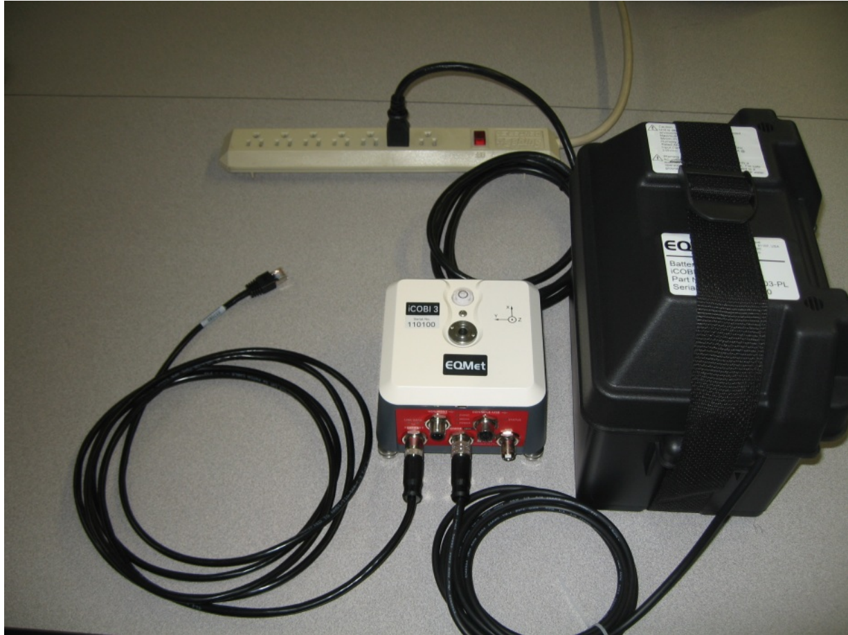
Figure 2.3: Bench setup for Top and Bottom Accelerograph
