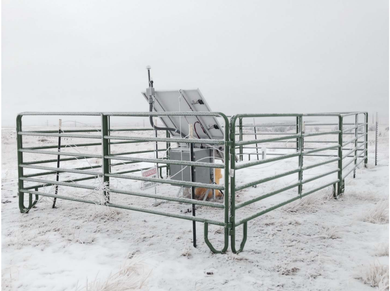
Figure 2: ARTIST station for temporary deployments with real-time communication
