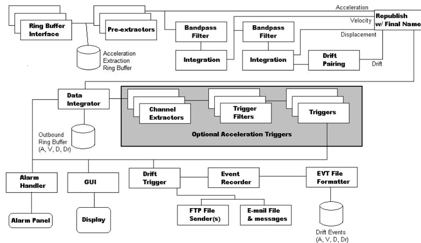
Figure 2.2. Data Flow in the OASIS processing.
