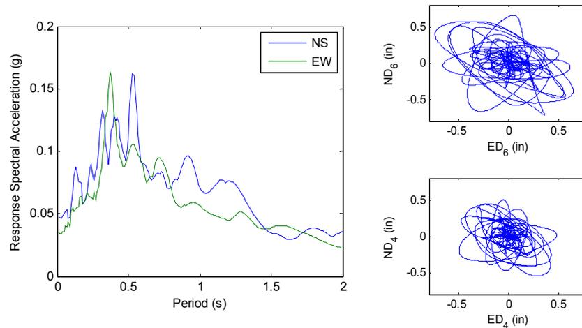
**Figure 3.5.** Response Spectral Accelerations from First Floor (left) and XY Particle Motion (right) where  $ND_x$  and  $ED_x$  are the  $x^{\text{th}}$  floor North-South and East-West Displacement respectively
