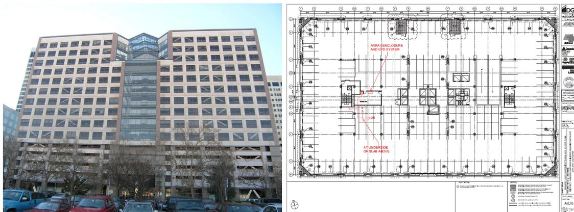
**Figure 3.3.** Caltrans District 4 Headquarters (left) and sample plan (right) showing sensor layout
