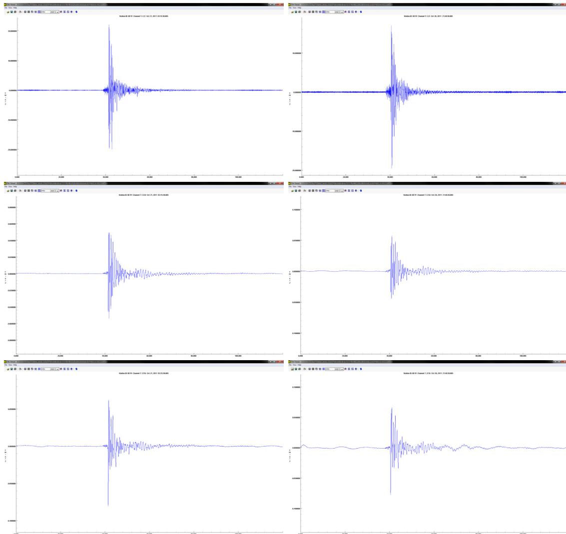
**Figure 3.1.** Sample data from one sensor during M4.0 (left column) and M3.8 (right column) earthquakes on October 20, 2011 near Berkeley, CA. Top, middle and bottom rows display acceleration ( $\text{cm/s}^2$ ), displacement (cm), and interstory drift (cm) versus time.
