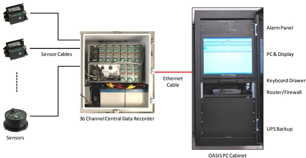
**Figure 2.1.** Kinometrics OASIS Seismic Monitoring System
