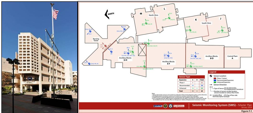
Figure 3.4. Naval Medical Center San Diego (left) and the SMS master plan (right) showing sensor layout
