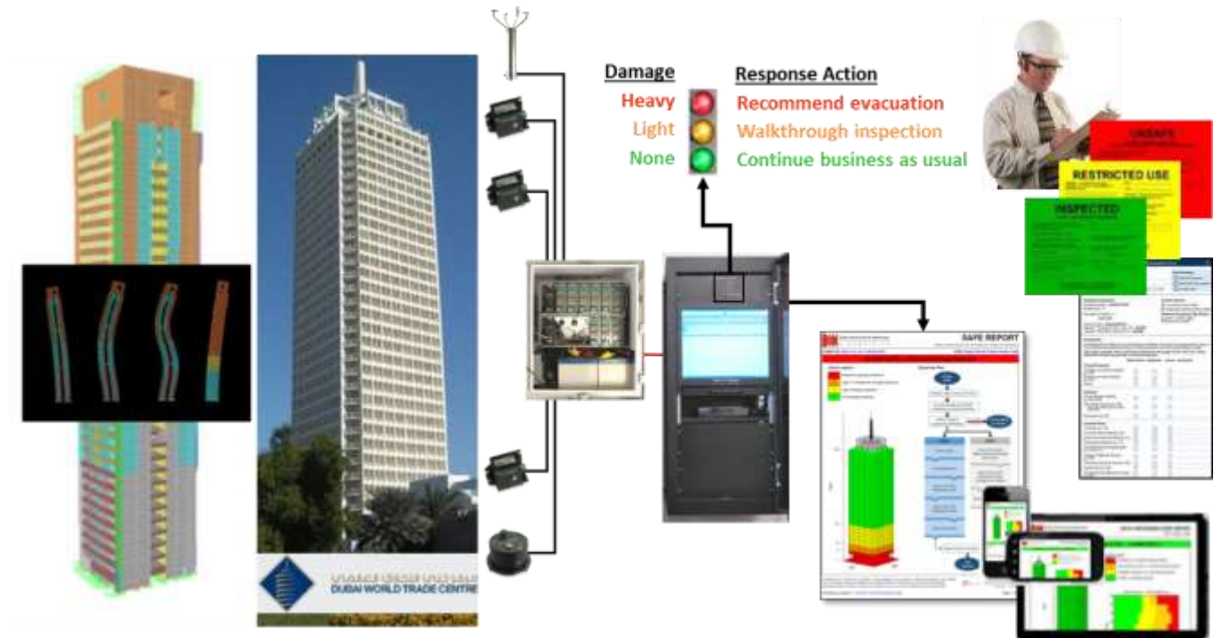
Fig. 3 – Conceptualization of OASIS and REAP integration
