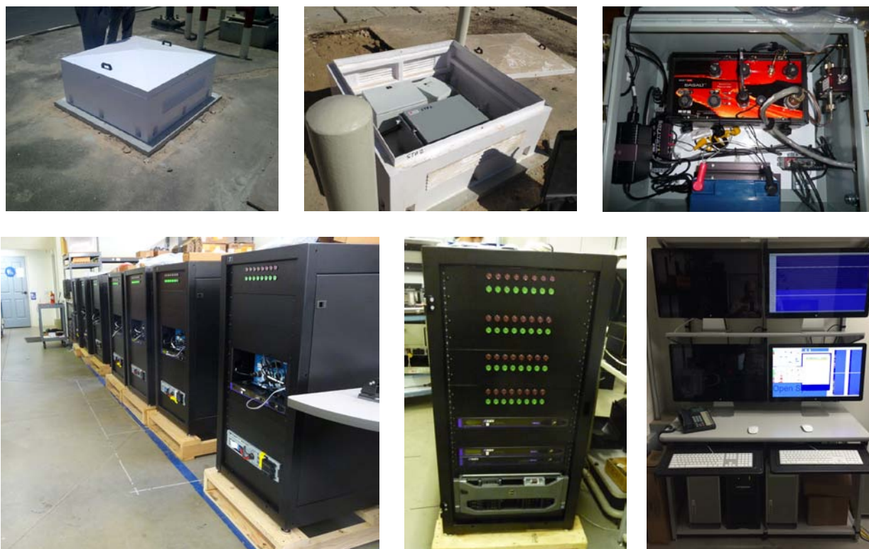
Figure 7. Photos of example earthquake alarm system components, clockwise from upper left: FFS, FFS with cover open, NEMA4 enclosure open showing Basalt datalogger and peripherals, display work station, central alarm controller and server, row of facility alarm controllers.
